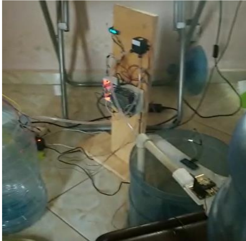
Figure 4.34: Assembled-Construction of Digital Water Level Control System
