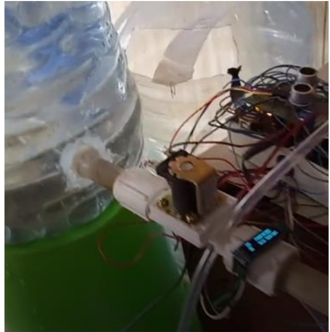
Figure 4.36: Pump stopping operation on the left and Solenoid valve connection on the right
