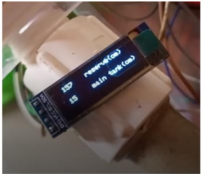
Figure 4.37: Solenoid valve allowing water to flow and the OLED reading at that instant respectively
