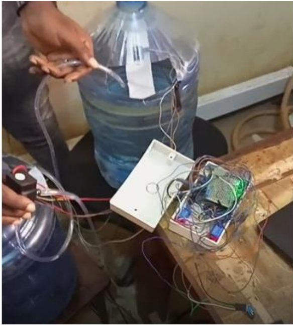
Figure 4.36: Pump stopping operation on the left and Solenoid valve connection on the right
