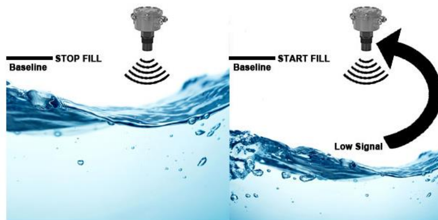
Figure 2.3: Ultrasonic Level Sensor water level controller [6]
