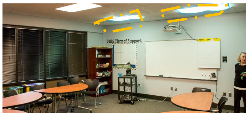
Figure 19: A typical classroom in Atlanta school for the deaf with cloth light diffusers (Hauan 2017).
