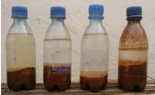
Figure 2-4: Dispersion test to check the gradation of the soil samples.
