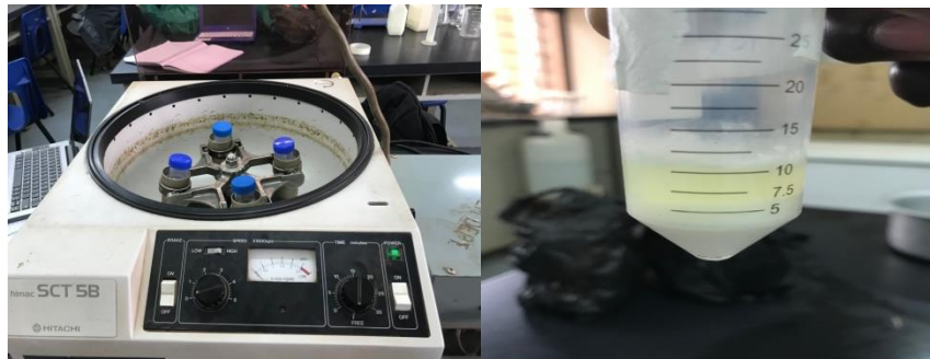
Figure 3.3: Centrifugation and whey separation
