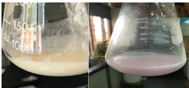
Figure 3.5: Color of yoghurt sample before and after titration
