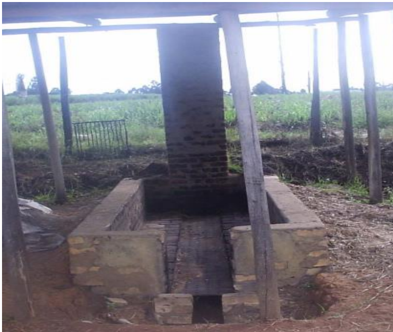
Figure 2 shows a brick-built kiln that was used to carbonize the dry bagasse.
