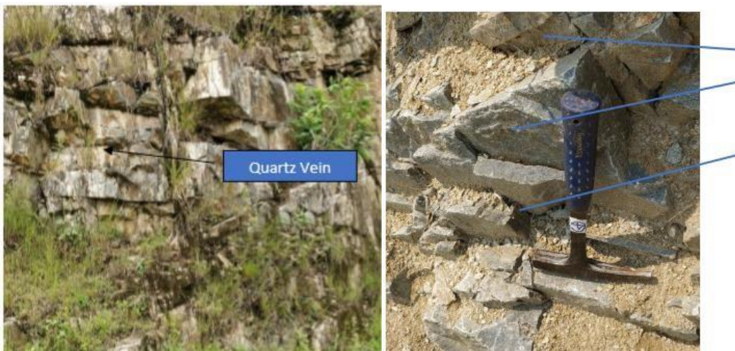
Figure 3. 2: A photograph showing quartz vein in a granitic gneiss in Kichwamba area (left)(186824/79600) and Granitic gneiss at quarry behind Kisegi hill(Right) (location: 192486/102083).(Heavily jointed, banded and foliated).
