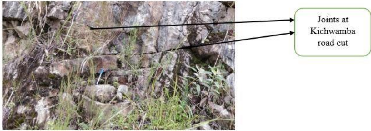
Figure 5. 1: A photograph showing a heavily jointed granite gneiss rock near Kichwamba Technical College. (location: 186824/79600, elevation: 1613m).
