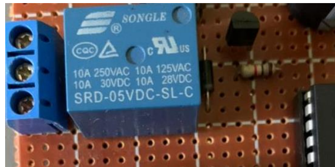
Figure 29: Relaying system on the device
