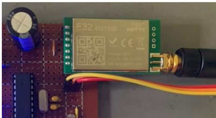
Figure 27: LoRa module on the device (Yaka meter side)
