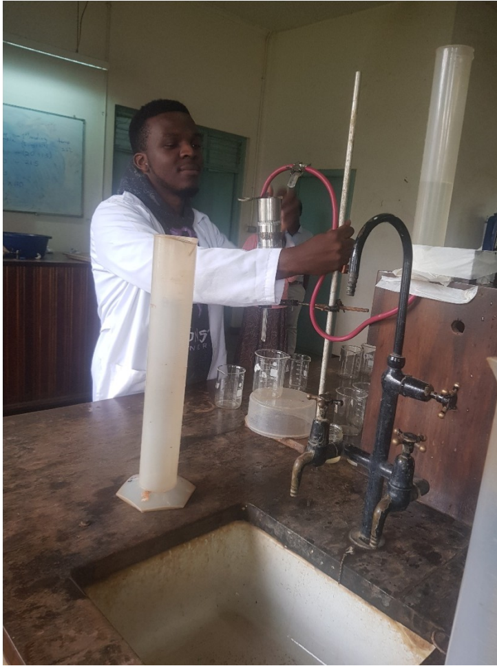
Figure 6. The student carrying out an experiment to determine saturated hydraulic conductivity of the soil.
