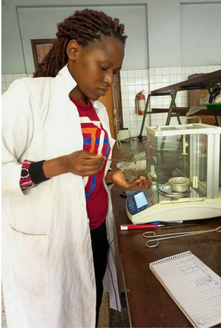
Figure 3- 1 measurement of substrates using a weighing scale before putting them in the oven for moisture content
