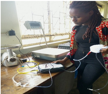
Figure A-4- 1: 0.8 Passing gas over the gas analyzer
