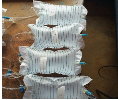
Figure 3- 6 Gas collected in urine bags to be taken for analysis
