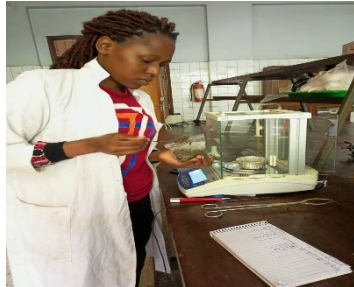
Figure A-2- 1: Measuring substrates for moisture content ,total solids and volatile solids characterization
