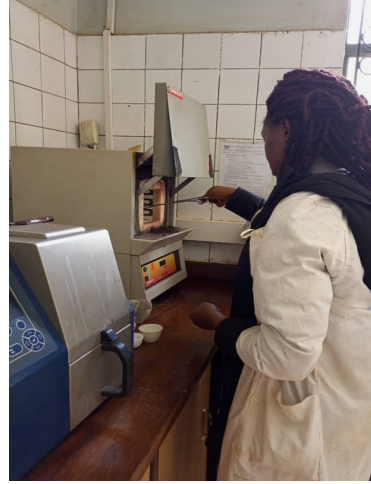
Figure 3- 3 Putting sample in the furnace to test for ash content and volatile solids
