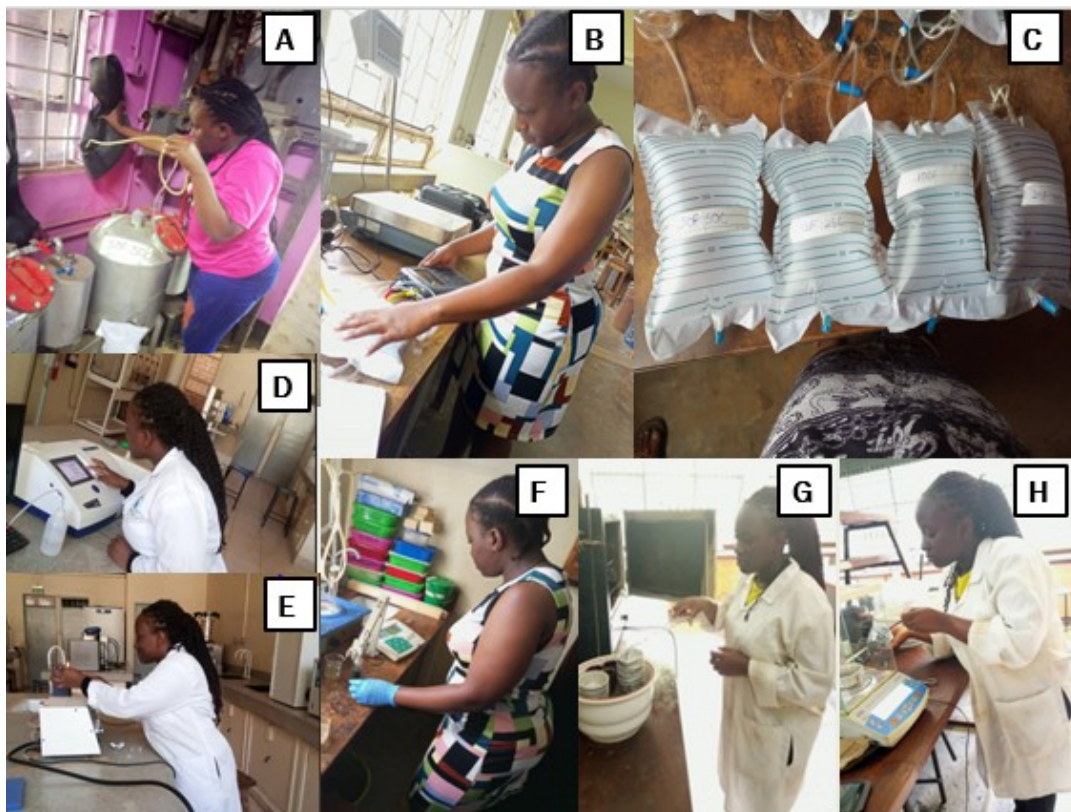
Figure 19: A-gas sample collection, B-Gas composition reading using a gas analyzer, C-Urine bags filled with gas samples, D & E Nutrient analysis, F-pH reading using a pH meter, G-Placing samples into the oven, H-Sample weighing.
