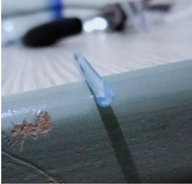
Figure 17 Filament with hollow cross section
