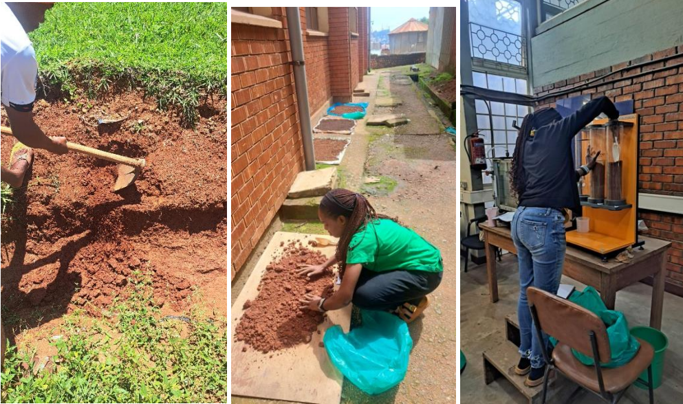
Figure 5- 1 Sample collection,drying and lab infiltration tests
