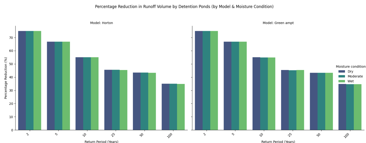
Figure 4- 8 Percentage reduction of runoff generated for detention ponds.
