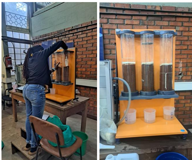
Figure3- 7 Lab infiltration tests and set up
