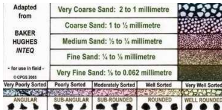
Figure13: showing the Grain size scale
