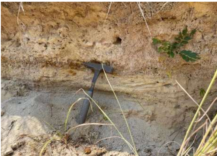
FIGURE 25: SHOWING AN INTERCALATION OF SAND AND CLAY BEDS WITH SOME GYPSUM
