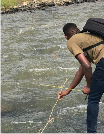
Depth measurement along points of the river
