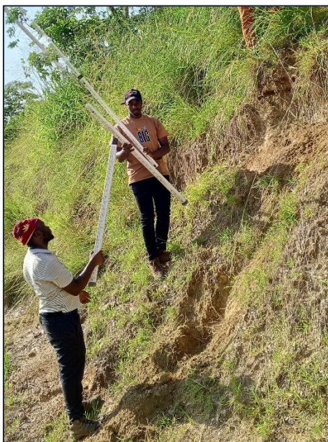
Figure 7. Illustrates the Jacob's Staff used to measure thickness of lithounits.
