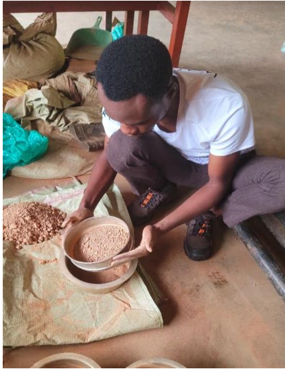
Figure 26. During sieving/preparing for LL test
