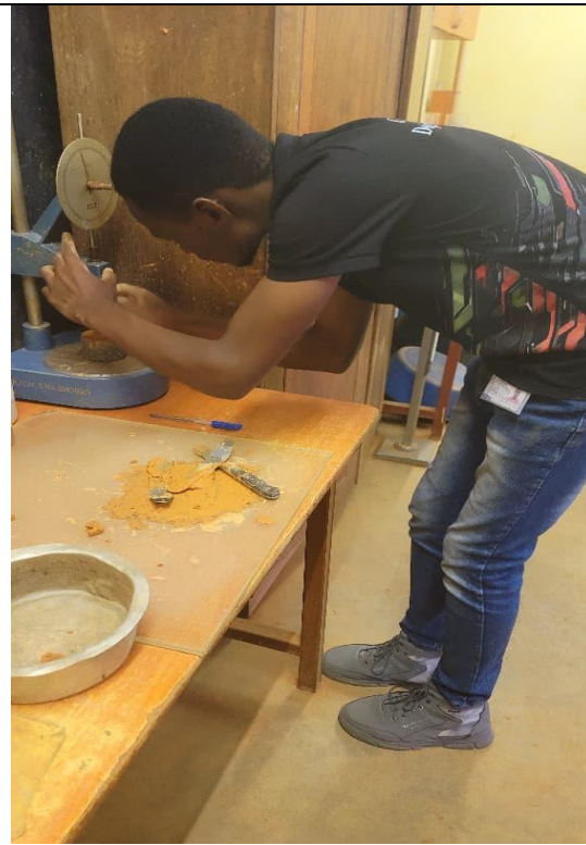
Figure 6. During cone penetration
