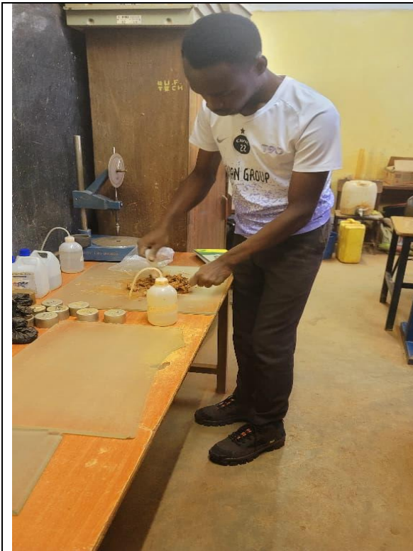
Figure 5. During mixing soil with distilled water
