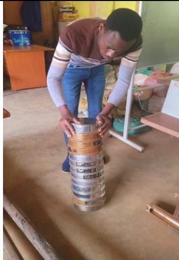
Figure 3. During sieve analysis
