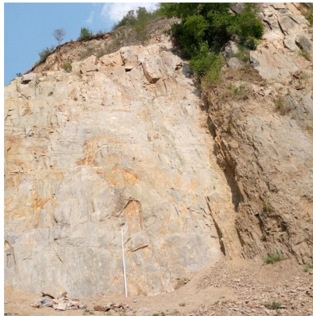
Figure 3.1: Large and highly fractured granitic gneiss outcrop at Kibuku quarry (192392E, 101800N, 668 m)
