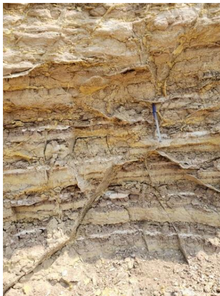
Figure 3. 4: Clay layers cemented by gypsum at the Kibuku road cut (192960E, 101767N, 746 m)
