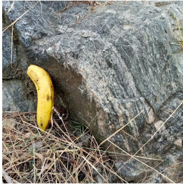
Figure 4.6: Foliation plane on granitic gneiss along a road cut at Kichwamba (186918E, 079296N, 1614 m).
