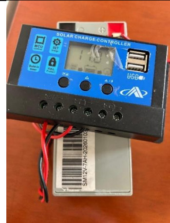
Figure 3-8 Solar charge controller and battery
