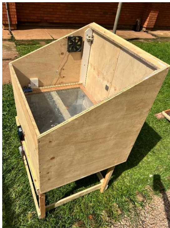
Figure 3-4 Constructed solar dryer
