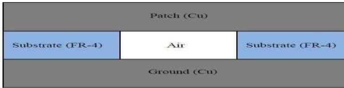
Figure 3: Side view of the proposed antenna
