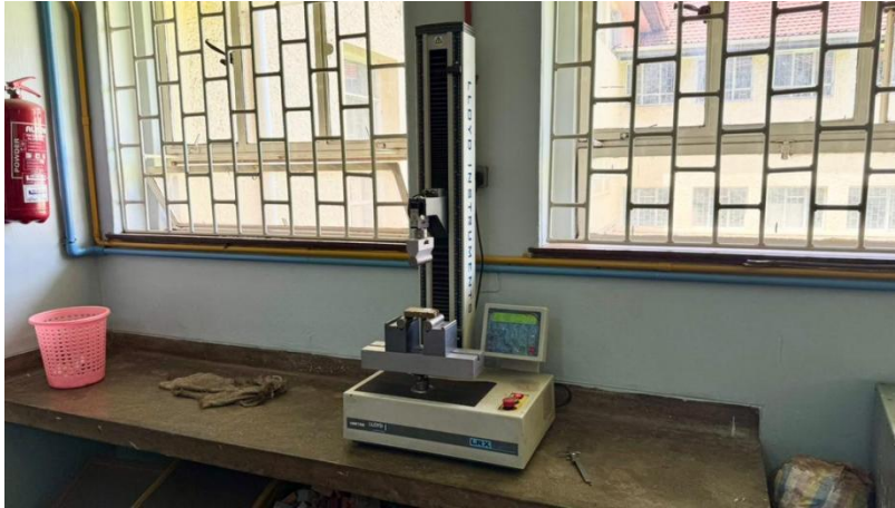
Figure A2. 7: Flexural strength testing
