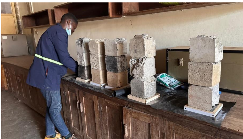
Figure A2. 3: uniform loading of samples
