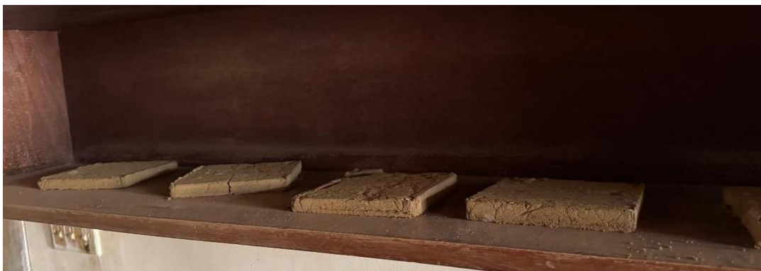
Figure 3-5: Curing of the sample boards in the laboratory
