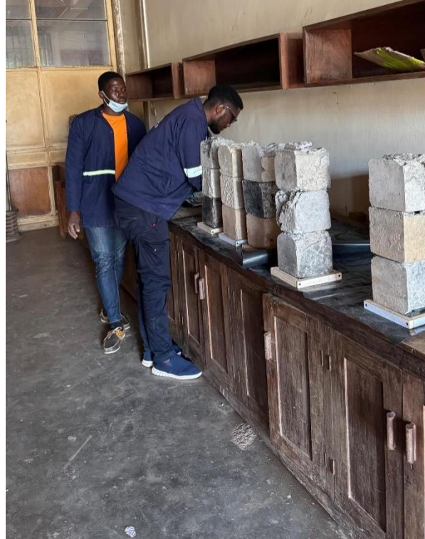
Figure 3-4: Sample under compaction using concrete blocks
