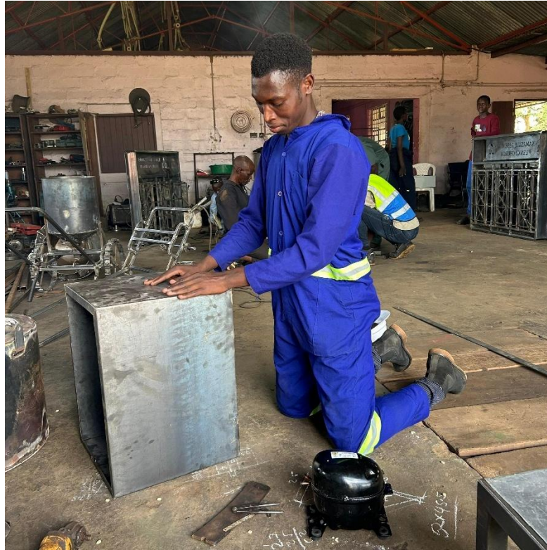
Figure 15: Outer cabinet shell – mild steel galvanised
