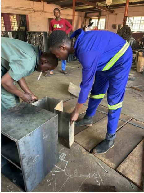
Figure 31: Inserting the inner cabin into the outside one
