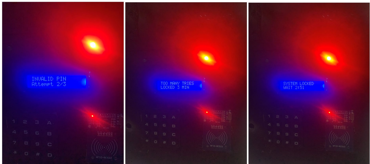
Figure 36: Wrong PIN/ RFID, 3 attempts, and a 3-minute countdown when the system was locked
