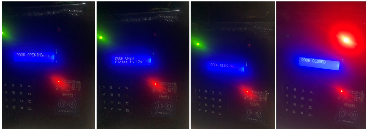
Figure 37: Door Opening and Closing Display
