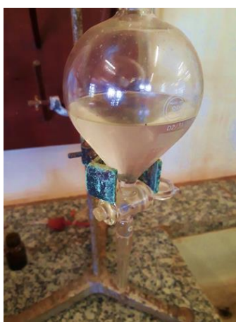
Figure 3.8: Upper layer of the product after tapping off the lower layer.
