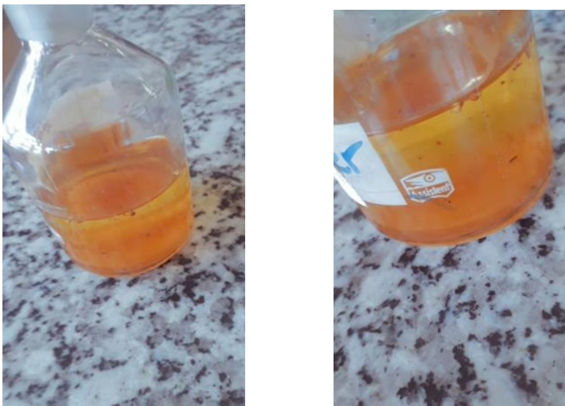
Figure 3.7: sample bottle with the collected oil from distillation residue showing a closer and distant view.
