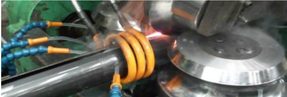
Figure 9: Induction welding process
