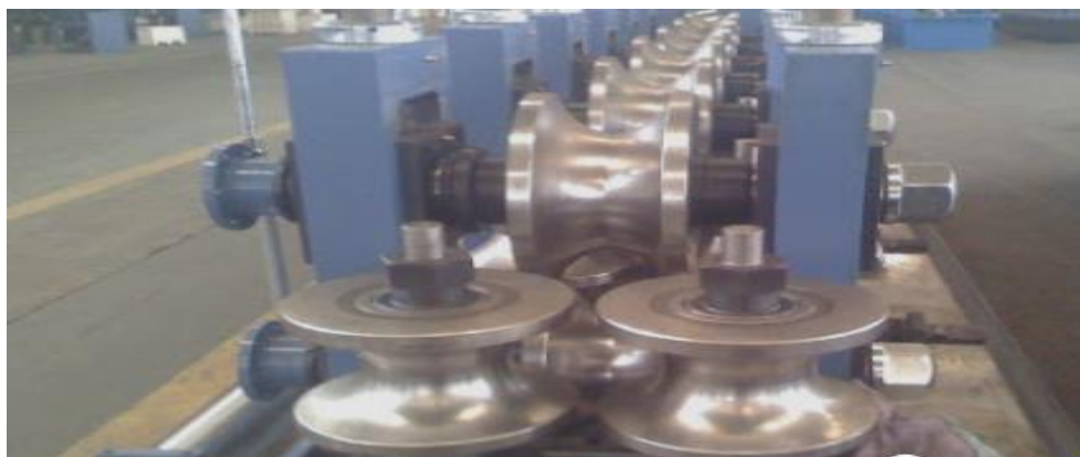
Figure 8: Tube forming process
