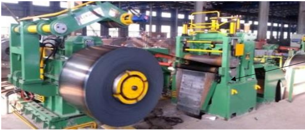
Figure 6: welding operation after de-coiling the slit
