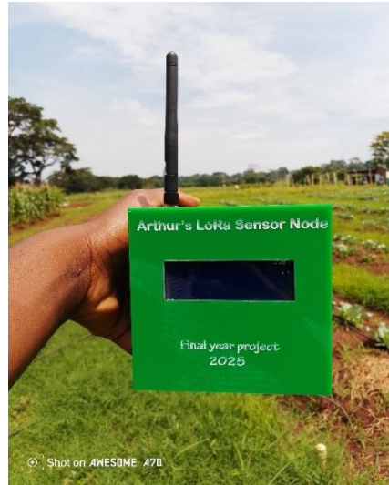
Figure 3.8: The acrylic housing
