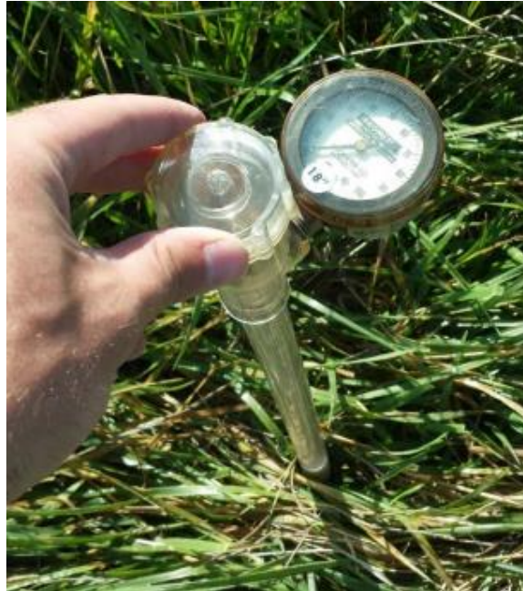
Figure 2.5: A tensiometer installed with a porous cup at the end (Sourced from: Sarkar et al., 2019)
