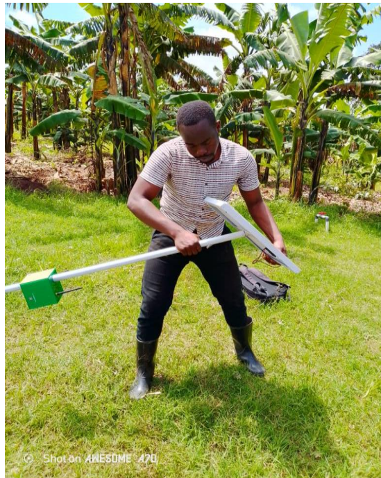
Figure 3.10: Setting up the solar panel on top of the rectangular frame situated at the top of the pole
