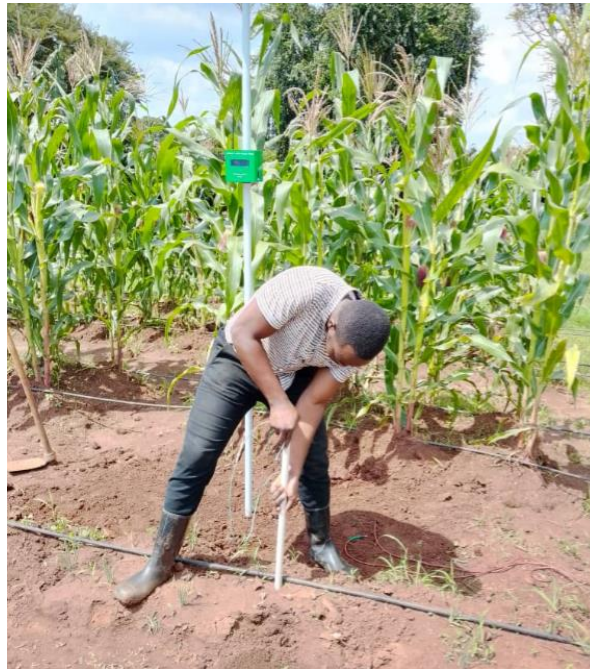
Figure 3.5: Installation of the watermark sensor in the active root zone of the crop.
