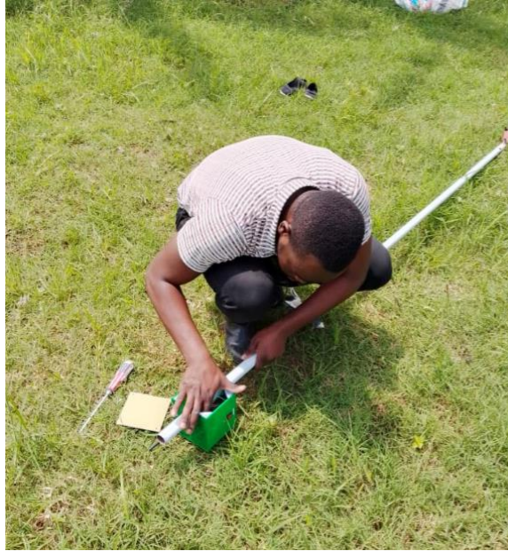
Figure 3.9: Inserting the acrylic casing on to the steel pole
