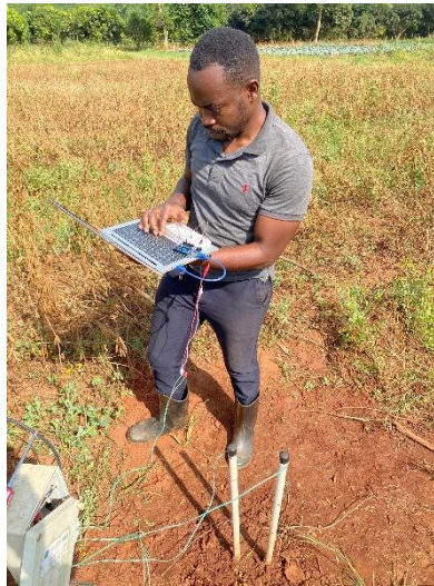
Figure 3.7: Reading of the soil water tension using my laptop in the Arduino IDE console.
